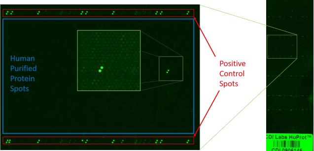
Figure 1: Magnified image of a monoclonal antibody -probed whole slide microarray showing localization of a mAb specific target antigen binding signal in duplicate. Positive controls are included in image.
